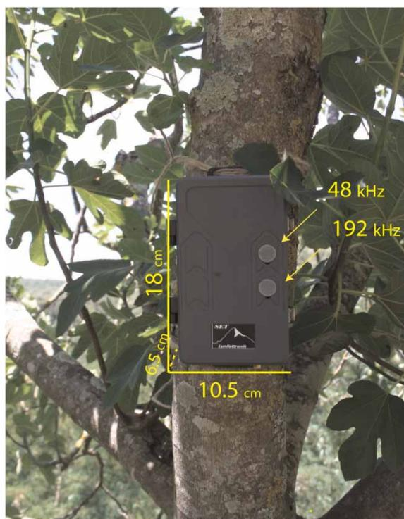
Figure 1. The Soundscape Explorer engineered by Lunilettronik ([www.lunilettronik.it](http://www.lunilettronik.it)) is a terrestrial (SE[T]) and aquatic (SE[A]) automatic sound recording (Farina et al., 2016, 2018).
